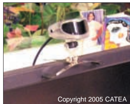
A head tracker receiver located on top of the monitor follows the movement of the user's head, which is then used to guide the cursor.
